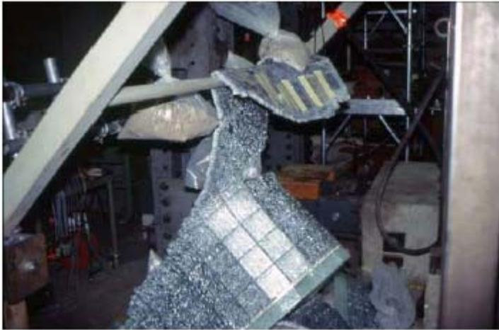
Fig. 5. Broken laminated glass.
